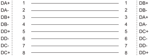
Straight-through Cable Wiring (MDI to MDI-X)
